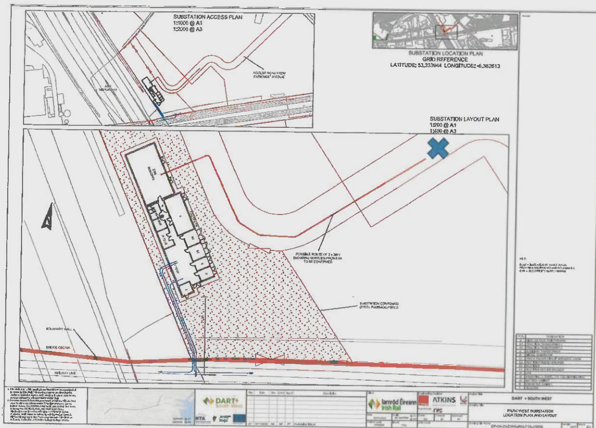
Figure 3: Extract from drawing submitted with Dart+ South West (Drawing title Park West Substation Location Plan and Layout - DP-04-23-DWG-RO-TTA-18856). Only a short section of electricity supply routing is shown on the drawing (terminating at the 'X' denoted by LDA).
